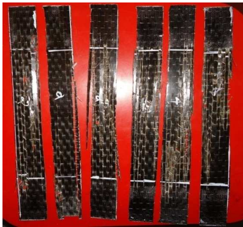
Figure 4: Failure Specimens of 90 0 Orientation Figure 5: Failure Specimens of 0 0 Orientation
